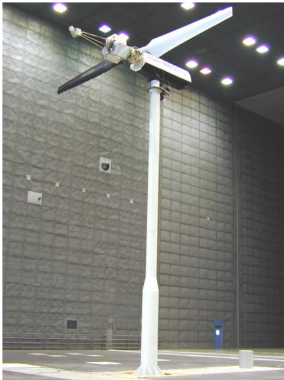
Figure 1. UAE wind turbine mounted in the NASA Ames 80 ft x 120 ft wind tunnel.
