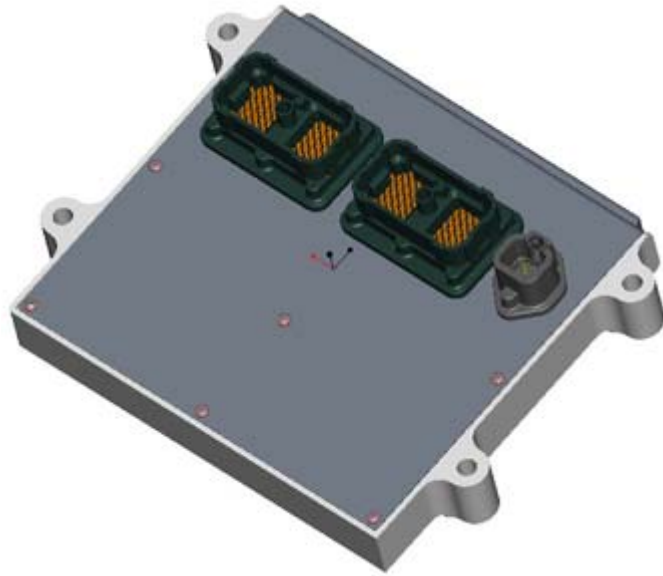
Figure (6): Layout of the new engine control unit (ECU)
