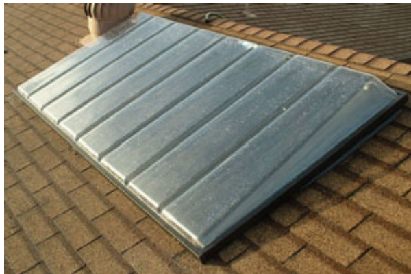
Fig. 2. DEG/SE glazed ICS on field test in Sacramento, CA.
