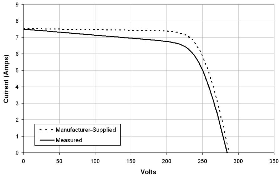
Figure 8. i-V curves comparing the manufacturer's curve to the measured curve and scaled to STC at 25°C (77°F) and 1000 W/m<sup>2</sup>.
