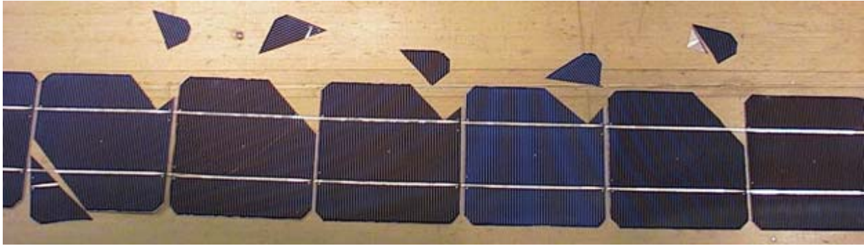
Figure 34 String of 220 \mu\text{m} cells soldered with 178 \mu\text{m} thick flat copper ribbon and flexed to show crack locations.
