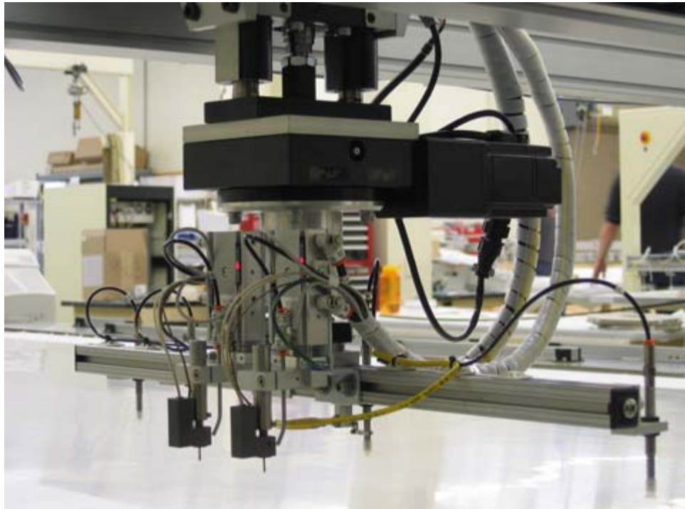
Figure 8 Robot end effector with soldering heads and vacuum pick-up arm.
