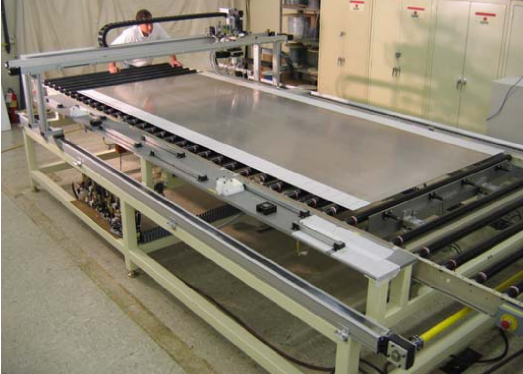
Figure 9 Module-size aluminum sheet on the automated busing system.
