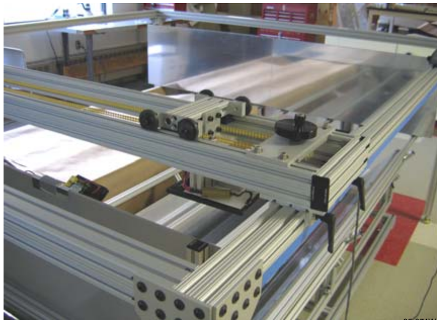
Figure 33 Monitor cell gantry for measuring light uniformity over a 2 m x 2 m test area.
