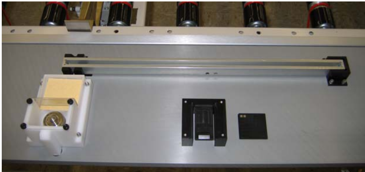
Figure 10 Bus ribbon tray (top), flux applicator (left), and diode pack retainer (center) on front tooling plate.
