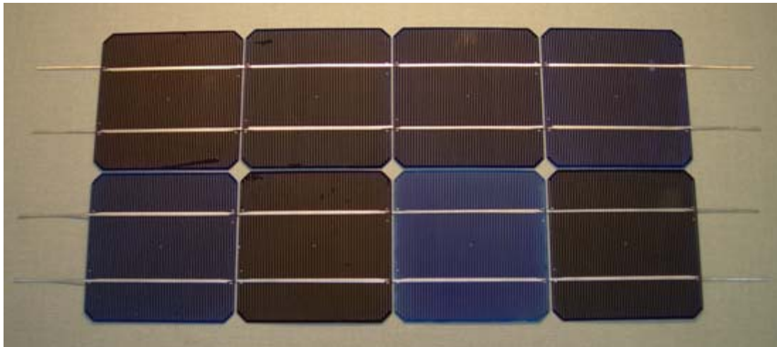
Figure 35 Cell strings made with 220 \mu\text{m} thin cells and 178 \mu\text{m} thick corrugated interconnect ribbons.
