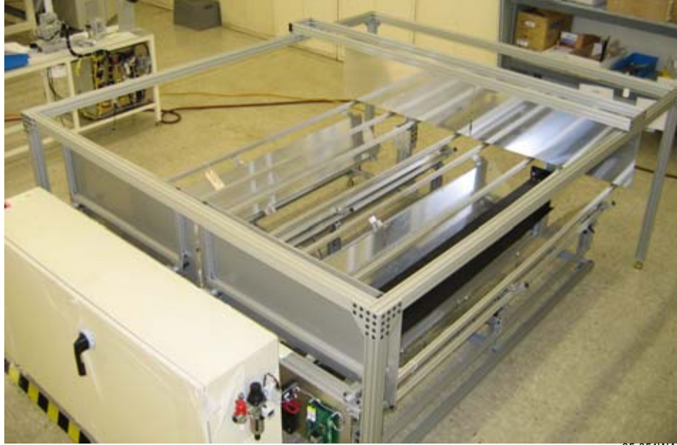
Figure 32 Solar simulator optical test bed with 2 m x 2 m test area.
