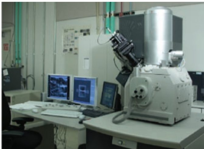
NREL's dual-beam focused-ion-beam workstation for fabricating microscopy samples and nanostructures.
