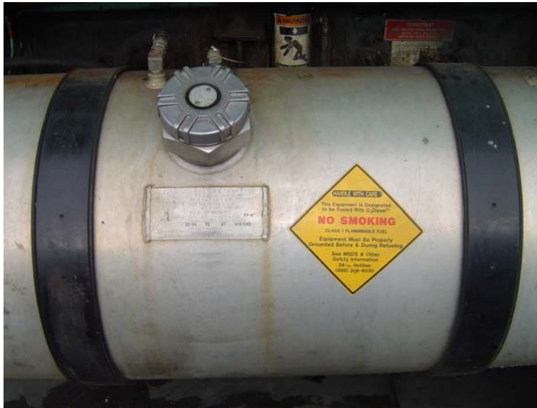
Figure 8. Fuel tank and O 2 Diesel sticker on refuse hauler at E.J. Harrison & Sons
