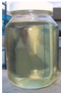
FIGURE 3A: EXAMPLE OF “CLEAR & BRIGHT” O 2 DIESEL™ MEETING THE FUEL’S SPECIFICATION.
