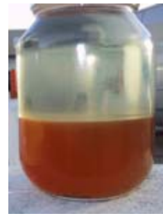
FIGURE 3B: EXAMPLE OF OPAQUE, CLOUDY APPEARANCE AND DISTINCT BROWN/BEIGE LINE OF PHASE SEPARATION DUE TO FUEL CONTAMINATION.
