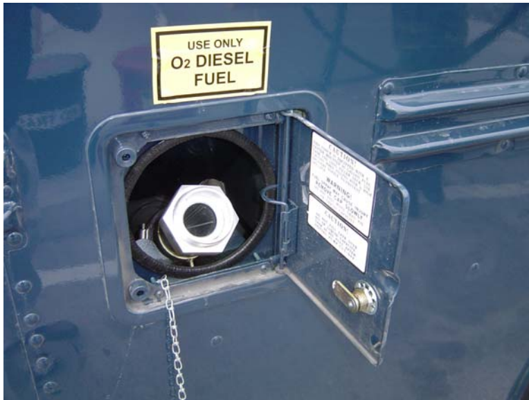
Figure 4. Flame arrester and O 2 Diesel sticker on Blue Bird bus at Nellis AFB
