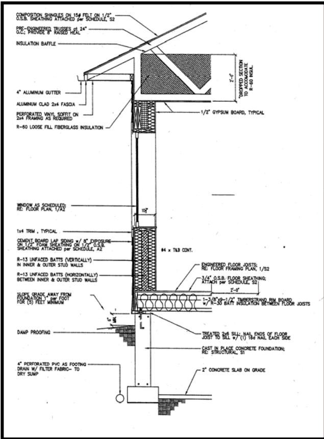
Fig. 2: Details of the double stud wall design
