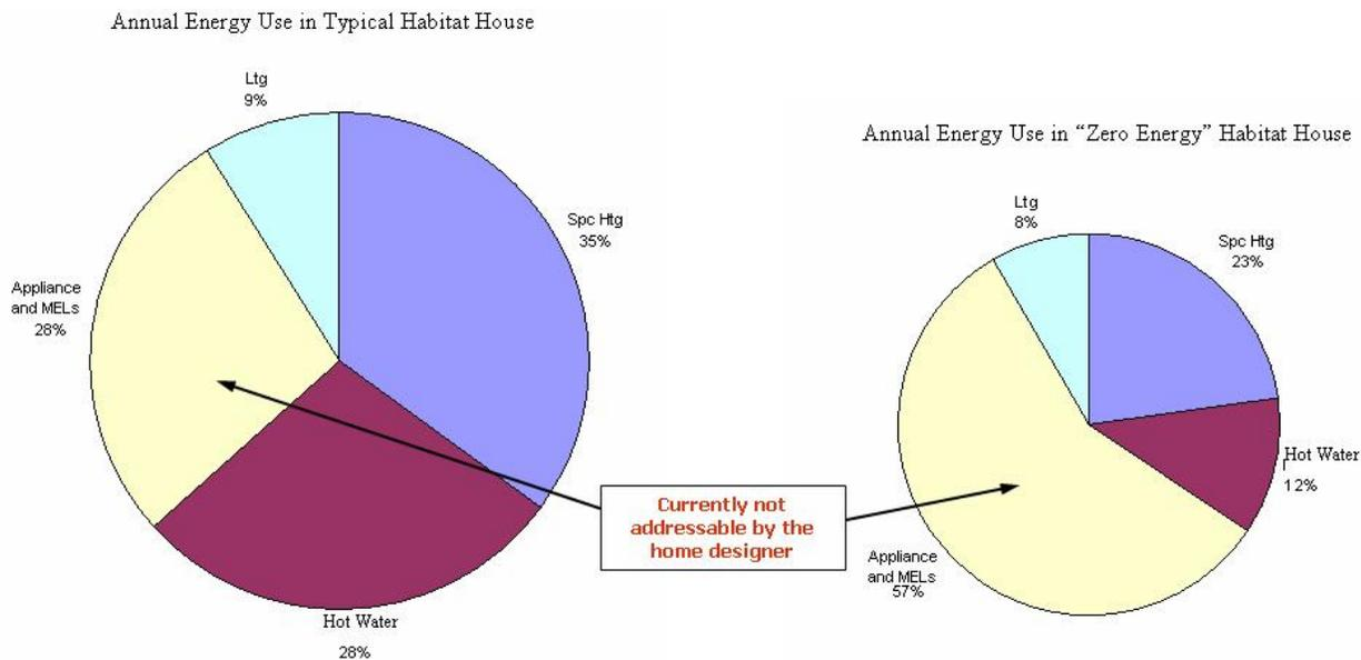
Fig. 6: Energy end uses for a typical design and the zero energy home.
