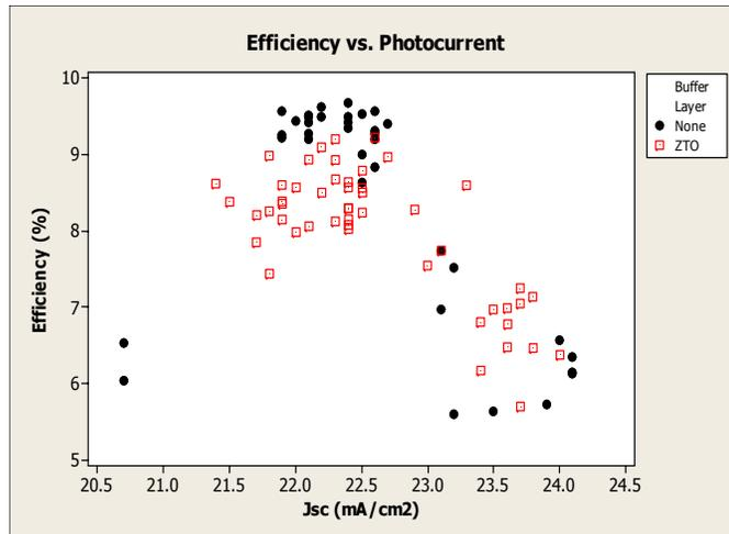
**Figure 2. Dependence of cell efficiency on  $J_{sc}$  for devices produced on various thicknesses of CdS - with and without a ZTO buffer layer<sup>4</sup>.**
