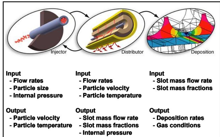
Figure 8. Primary elements of the distributor simulation model developed by CSM researchers.
