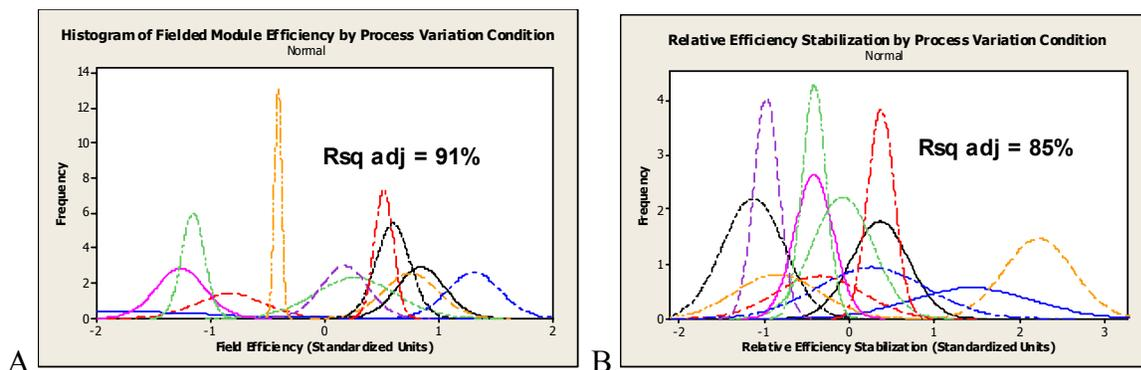
**Figure 16** Normalized histograms showing distribution of **A. Fielded module baseline efficiency** and **B. Relative change in efficiency of fielded modules over time** for each of 12 process conditions of a designed experiment. Adj Rsq is a measure of the percentage of overall variation that is explained by process condition. Standardized Units are average divided by standard deviation. Positive values of Relative Efficiency Stabilization indicate smaller changes in relative performance.
