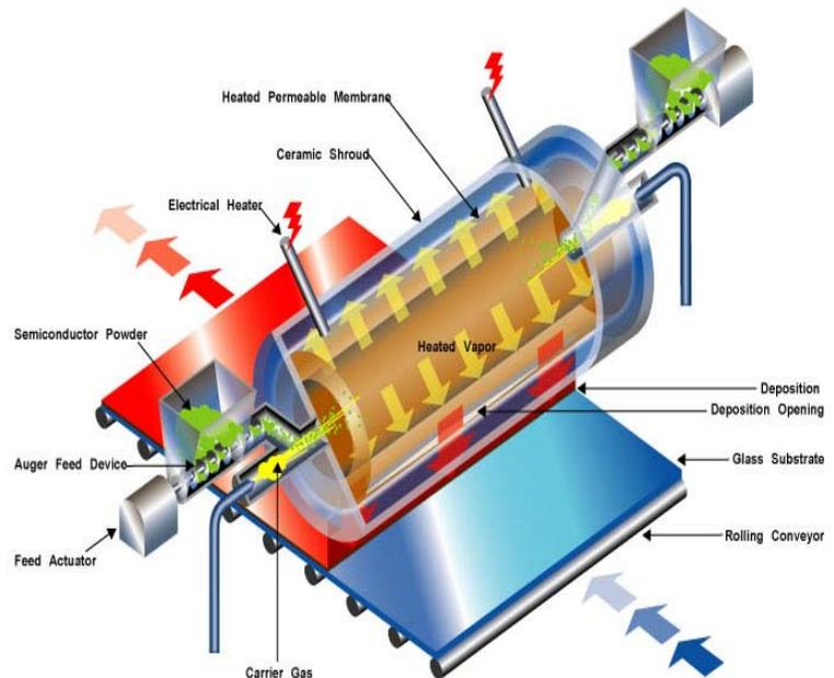
Figure 4. Conceptual drawing of First Solar proprietary VTD system. First Solar's High Rate Vapor Transport Deposition system was awarded an IR&D 100 award in 2003.
