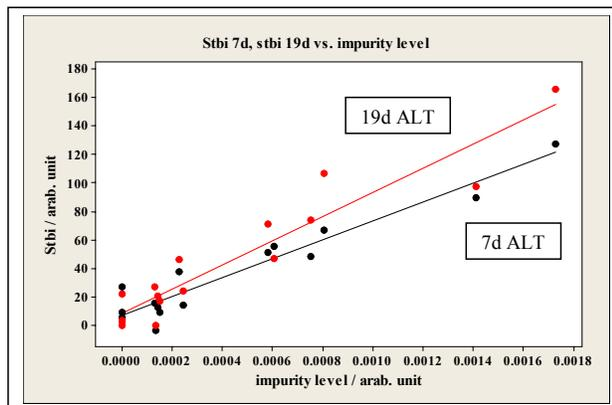
**Figure 12. Relative efficiency as a function of added impurity level of devices after 7 and 19 days light soak at 120 C.**
