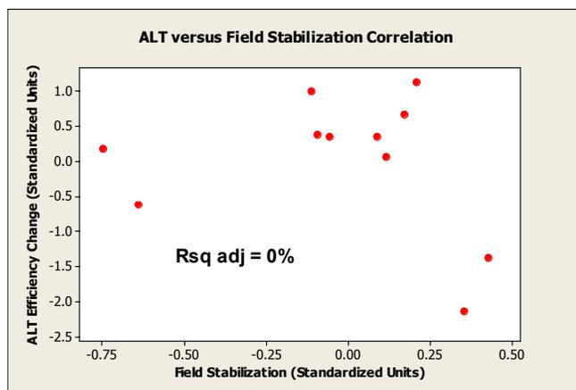
**Figure 17.** Correlation between change in performance as indicated by ALT and observed change in field data. As indicated by R-sq(adj) there is no indicated correlation between ALT and Field Stabilization values.
