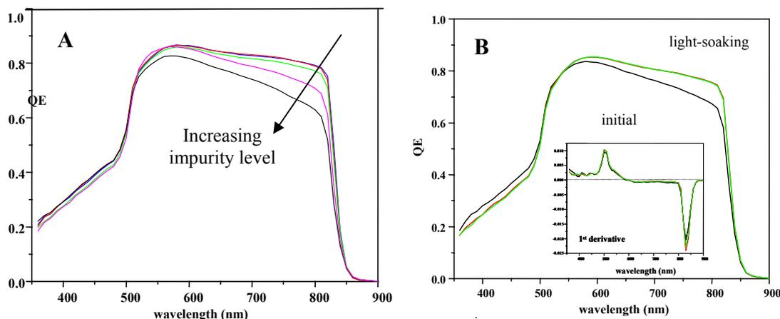
**Figure 13. A. Initial quantum efficiency for devices with varying impurity levels and B. Quantum efficiency improvement after light soaking at 120 C for 7 and 19 days.**
