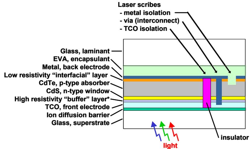
Figure 1. Schematic cross section of First Solar polycrystalline thin film CdTe PV module showing films and interconnect scribes. The TCO, buffer layer, and CdS window films are collectively referred to as the Advanced Front Contact Window layer (AFCW).
