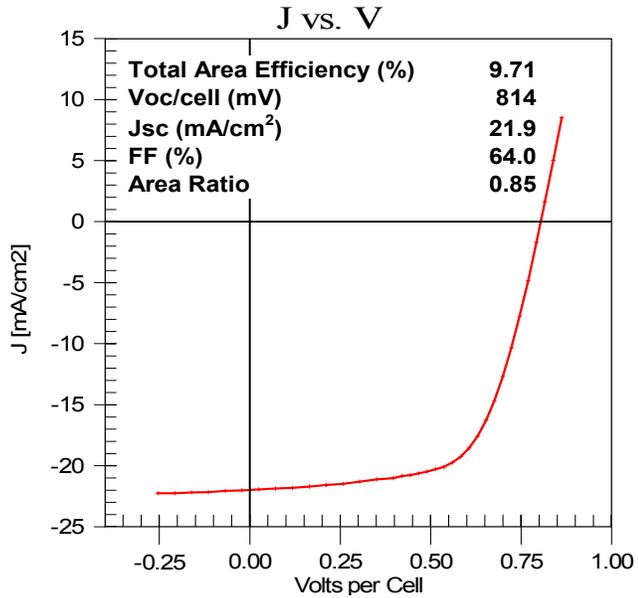
Figure 3. Champion 7200 cm<sup>2</sup> module achieved using a buffer layer.
