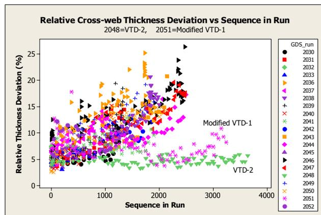
**Figure 5. Cross-web thickness uniformity of CdTe films deposited with different distributors. Relative deviation is lower and remains constant throughout a 3600 plate run with the VTD-2 distributor design.**
