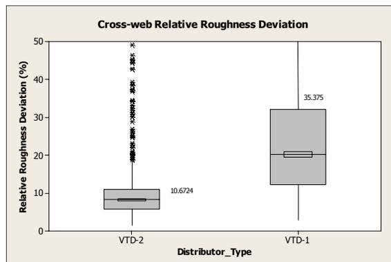
**Figure 7. Box plot of relative cross web surface roughness deviation.**
