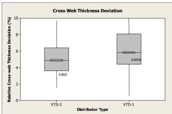
**Figure 6. Box plot of relative cross-web thickness deviation. VTD-2 distributors average about a 5% cross-web thickness deviation.**
