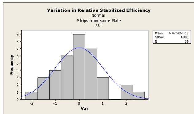
**Figure 15. Variation of relative baseline performance as predicted by curve-fitting for strips from the same plate that were stressed at elevated temperature. Variation is defined as  $100 \times (P - P_{avg}) / P_{avg}$ , where P is the predicted value and  $P_{avg}$  is the average of P on one plate.**
