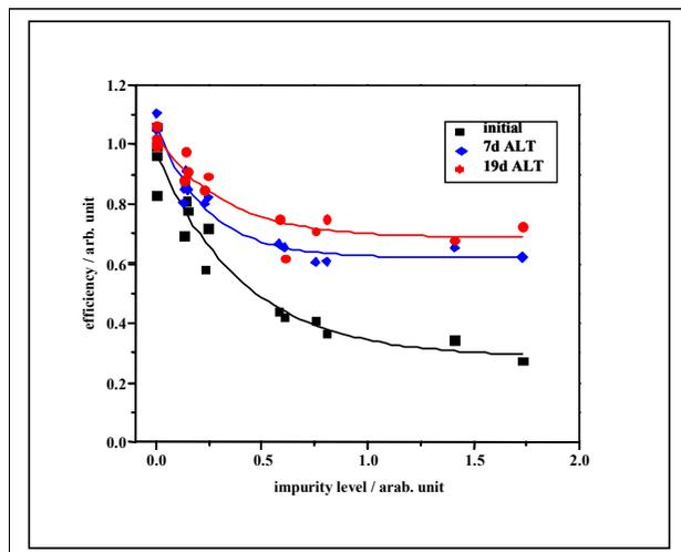
**Figure 11. Representative data showing relative changes in efficiency with lightsoak for devices with and without intentionally introduced impurities. Note that absolute efficiency was higher for devices without impurities.**
