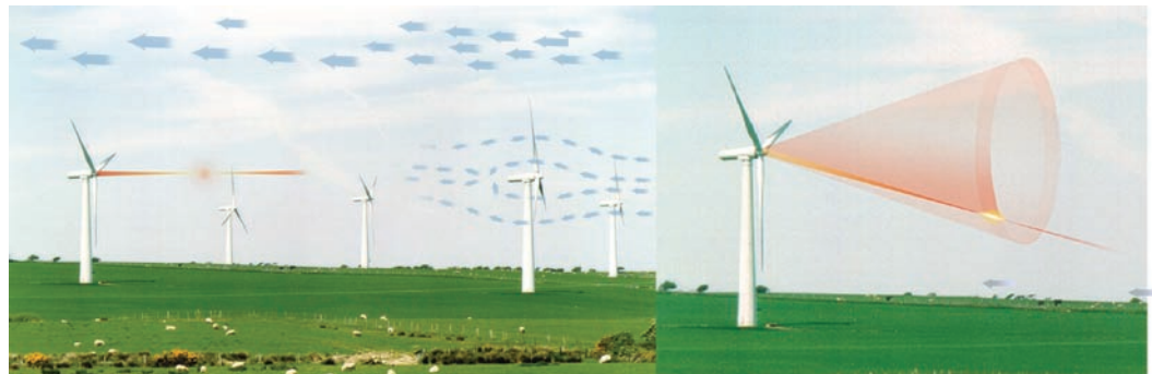
Examples of LIDAR scanning options, showing hub-mounted staring scheme and hub-mounted conical scan.
