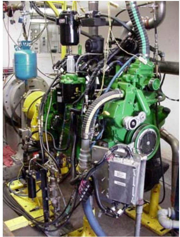
Photos 3-1 and 3-2. John Deere 8.1L deterioration factor engine installed on laboratory dynamometer at SwRI
