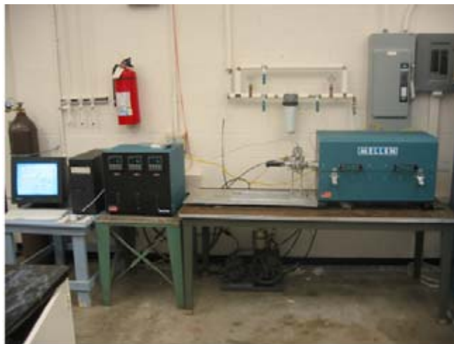
Figure 14: The entire system (LPD reactor and DTA) in its final version at the end of the project.
