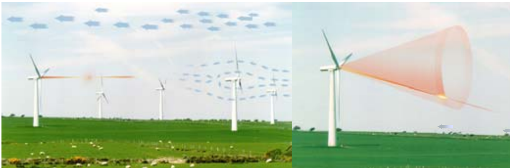
Figure 8. Examples of scanning options, showing hub-mounted staring scheme and hub-mounted conical scan
