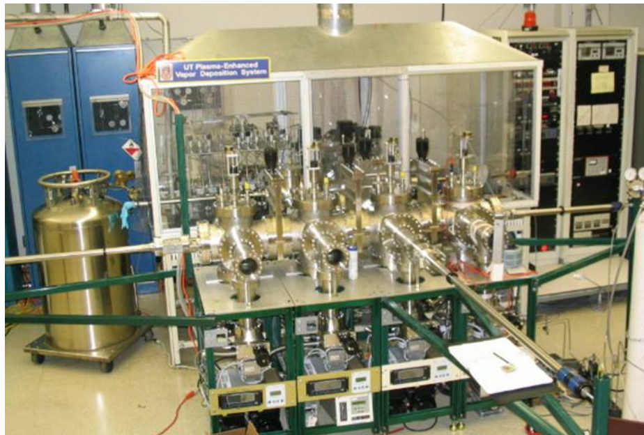
Fig. 15-5: Photo of the entire system with nine chambers--3 PECVD, 1 HWCVD, 4 Sputtering, and 1 Load lock chambers.
