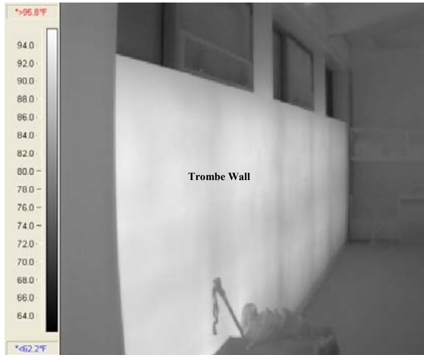
Figure 9. Interior infrared picture of Zion Trombe wall December 16, 8:30 p.m.
