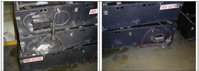
Figure 6. Normal battery tray (left) and tray with a corroded cable (Source: NREL)
