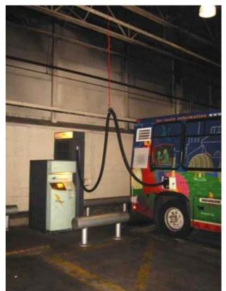
Figure 15. IndyGo Ebus at Charging Station (Source: NREL)
