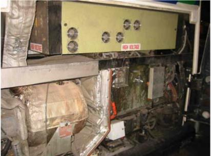
Figure 14. Capstone MicroTurbine Assembly (Source: NREL)
