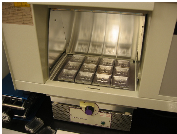
Fig. 2. Solar Matched Stress Test System ▪ 96 sample capability ▪ 1500 hour continuous runs ▪ Continuous temperature monitoring ▪ V_{oc} bias testing ▪ AM 1.5 calibrated solar spectrum.
