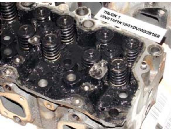
Figure 9. Mack No. 1 B20 Valve Deck Sludge Accumulation
