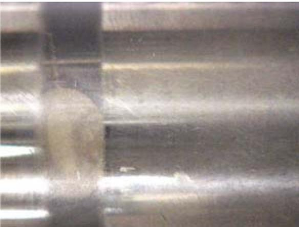
Figure 8. Mack No. 3 Diesel Oil Pump Pressure Relief Valve Piston Wear
