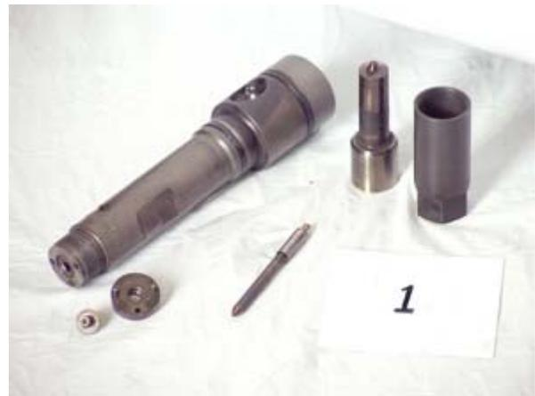
Figure 11. Mack No. 1 B20 Worn Fuel Injector Nozzle Disassembled
