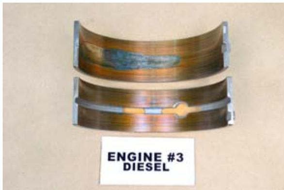
Figure 14. Ford No. 3 Diesel Main Bearing Failure
