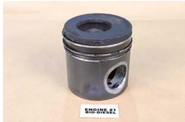
Figure 13. Ford No. 1 B20 Piston Carbon Deposits
