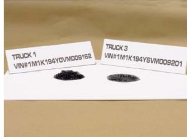
Figure 10. Cylinder Head Sludge Comparison (Mack No. 1 B20 vs. Mack No 3. Diesel)
