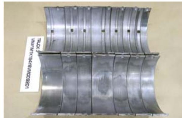
Figure 6. Mack No. 3 Diesel Main Bearing Wear
