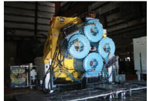
This Clipper 2.5-MW drivetrain underwent dynamometer testing at the National Wind Technology Center.
