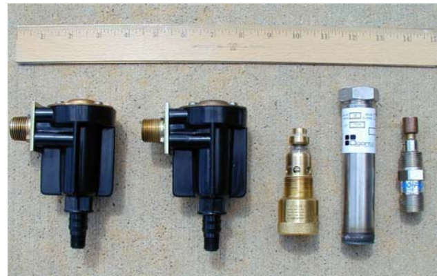
Fig. 3: Five freeze protection valves. From left to right: Dole/Eaton FP-45, Dole/Eaton FP-35, Therm-Omega-Tech IC/FP-35, Ogontz F 35 BDT, and ProFlo V243T. Only the first three were tested.
