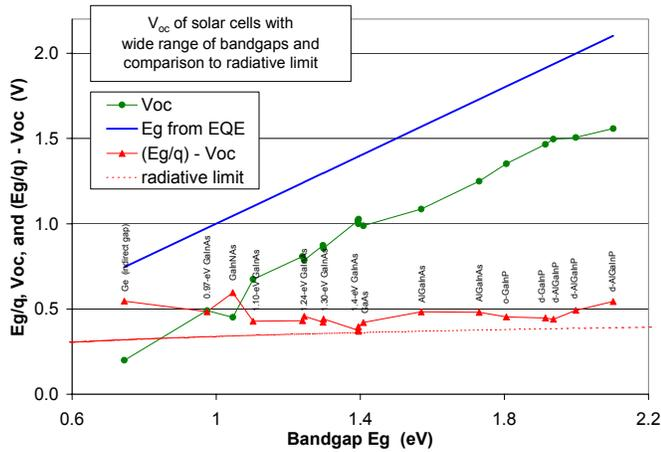
Figure 7. Experimental  $V_{oc}$  for a wide range of single-junction solar cell bandgaps, from 0.67 to 2.1 eV, showing that the bandgap-voltage offset,  $(E_g/q) - V_{oc}$ , is roughly constant over this range as predicted from theory. The value of this offset approaches the radiative limit for some solar cell materials.
