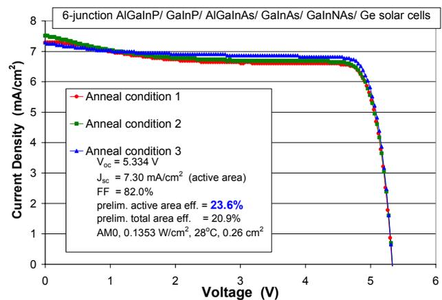
Figure 10: Illuminated current-voltage characteristics for 6-junction AlGaInP/ GaInP/ AlGaInAs/ GaInAs/ GaInNAs/ Ge solar cells, with an active  $\sim 1.1$ -eV GaInNAs subcell 5, with  $V_{oc}$  over 5.3V.
