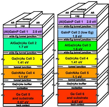
Figure 3. Cross-sections of 5- and 6-junction cells.
