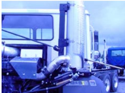
FIGURE 27. THREE-WAY CATALYST CHASSIS MOUNT LOCATION
