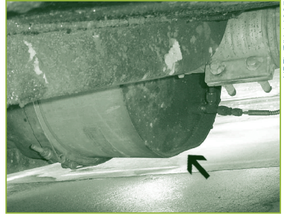
Figure 4. Low clearance of the CCRT resulted in damage
