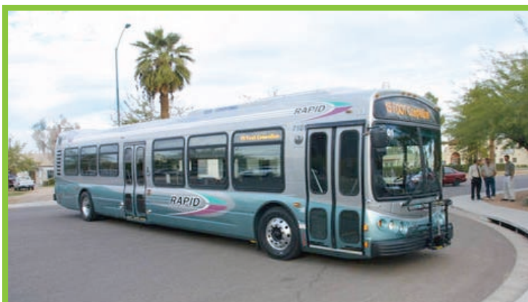
Figure 1. Liquefied Natural Gas Bus Operated by Arizona's Valley Metro NREL/PIX 12534
