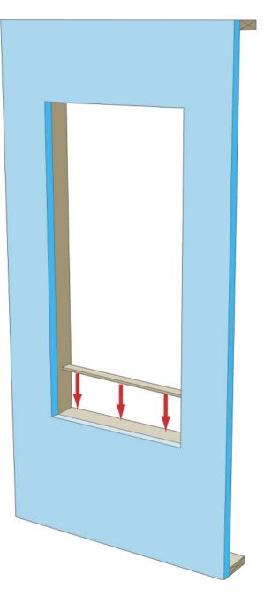
Apply first piece of adhesivebacked sill flashing; apply second piece of adhesivebacked sill flashing
