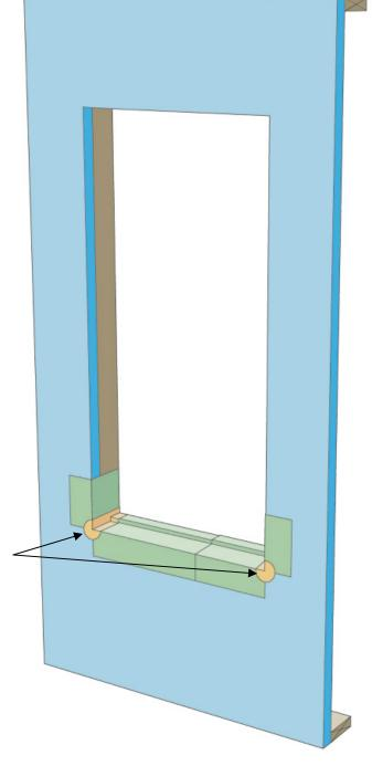
The yellow material in this illustration shows where the corner flashing patches should be applied in order to cover the holes at the folds in the underlying flashing.
