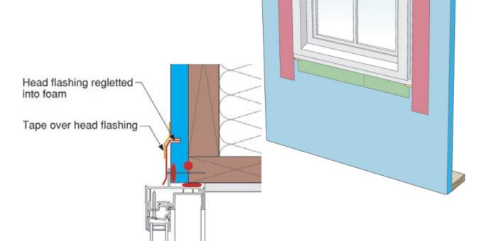
Tape head flashing; air seal window around entire perimeter on the interior with sealant or nonexpanding foam
