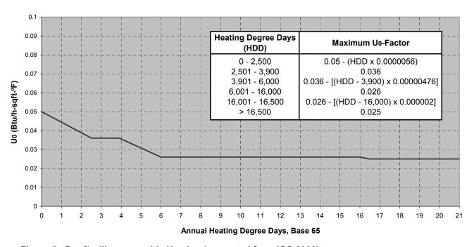
Figure 5. Roof/ceiling assembly U-value (excerpted from ICC 2003)
