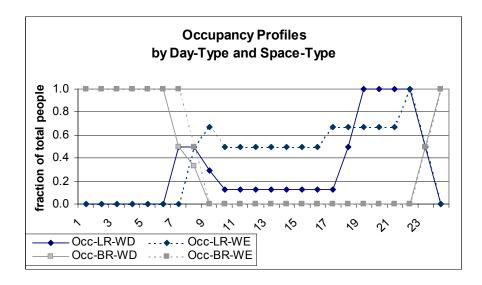
Figure 22. Detailed hourly load profiles resulting from occupants being in different parts of the house on weekdays (WD) and weekends (WE)
