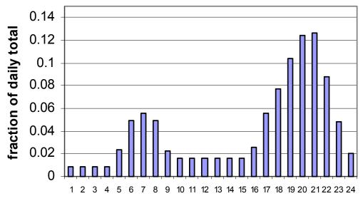
Figure 12. Interior lighting profile (built up from detailed profiles)
