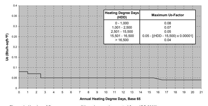
Figure 1. U-value of floor over unconditioned space (excerpted from ICC 2003)
