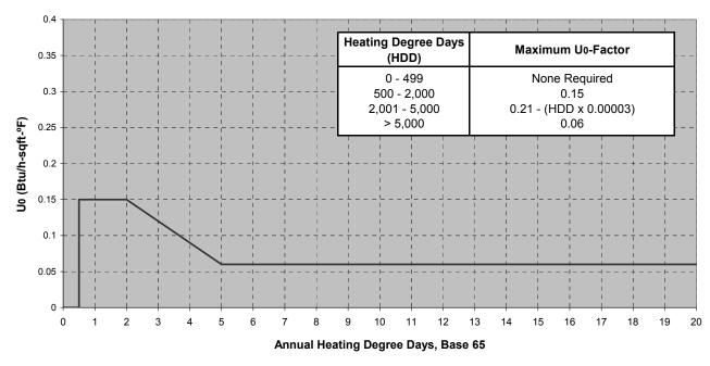
Figure 2. Unvented crawl space wall U-value (excerpted from ICC 2003)
