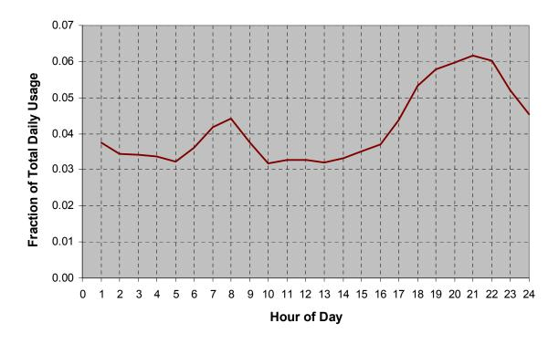
Figure 20. Other appliance and plug load normalized energy use profile
