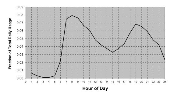
Figure 9. Combined domestic hot water use profile
