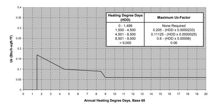
Figure 3. Basement wall U-value (excerpted from ICC 2003)
