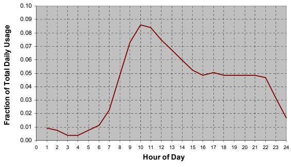
Figure 16. Clothes washer normalized machine energy use profile (Pratt 1989)
