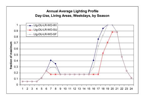
Figure 13. Example of a detailed lighting profile (expressed as fraction of peak daily lighting energy)
