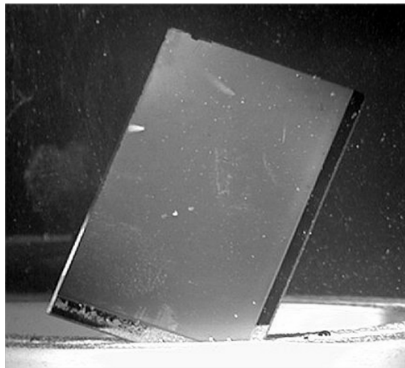
Figure 5. Elimination of adherent bubbles upon addition of surfactant to bath
