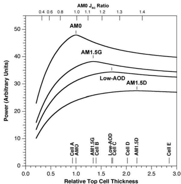
Fig. 1. Calculated power produced by a GaInP/GaAs/Ge triple-junction cell as a function of  $t_{top}$  for Air Mass 0, 1.5 Global, 1.5 Direct, and Low Aerosol Optical Depth standard reference spectra. Relative  $t_{top}$  values are shown, normalized to the optimal AM0  $t_{top}$ . Although the power produced by a GaInP/GaAs tandem cell will be less, the optimal  $t_{top}$  for any given spectrum will not change. Approximate  $t_{top}$  values for cells A - E are indicated.
