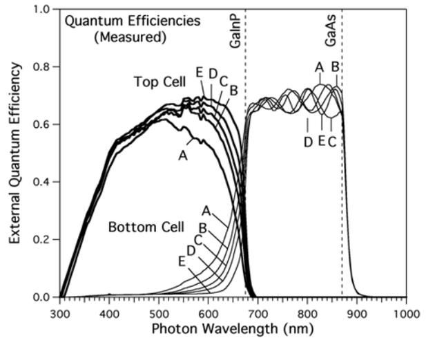
Fig. 4. Measured external quantum efficiencies for the top and bottom cells. Cell C is represented by C2. (Cell C1 data is not shown.) A small non-physical sub-band-gap top cell response was removed by smoothly setting the top cell QE to zero for wavelengths greater than  $\sim 700$  nm.
