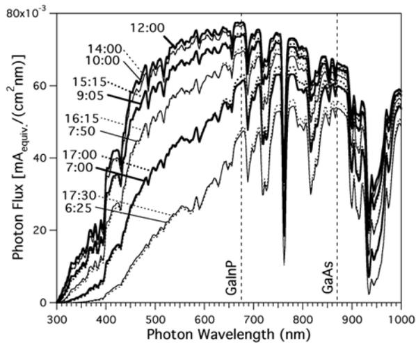
Fig. 3. Measured direct spectra labeled by time of day during the test day. The photon flux is expressed as mA equivalent for 100 percent conversion of photons to photocurrent, per  $\text{cm}^2$  area and nm of wavelength. The GaAs and GaInP band gaps are indicated with vertical dashed lines. Morning spectra are plotted with solid lines. Afternoon and evening spectra are plotted with dashed lines.
