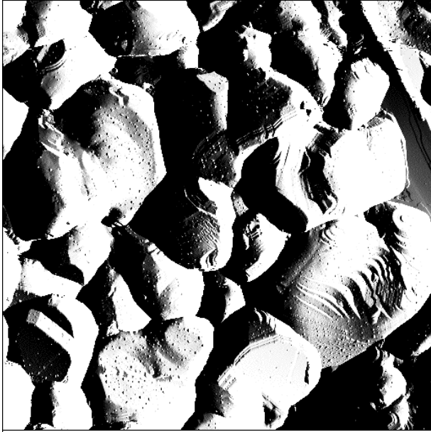
0 5.00 \mu\text{m} Fig. 2b. AFM image of \text{CdCl}_2 -treated LT CdTe sample deposited on glass/ \text{SnO}_2 / \text{CdS} / \text{NaF} in \text{He}/\text{O}_2 ambient.
