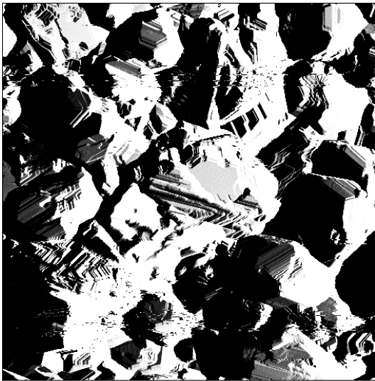
0 5.00 \mu\text{m} Fig. 2a. AFM image of as-deposited LT CdTe sample deposited on glass/ \text{SnO}_2 / \text{CdS} / \text{NaF} in \text{He}/\text{O}_2 ambient.
