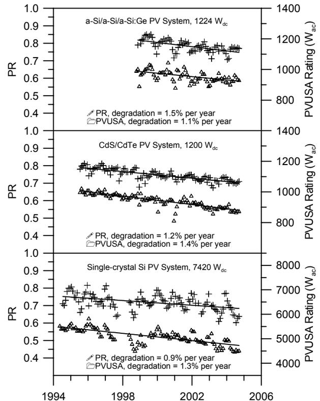
Fig. 6. Long-term degradation rates for three PV systems at NREL from monthly values of PR and PVUSA ratings. Upper regression lines from monthly PR values shown by + symbols. Lower regression lines from monthly PVUSA values shown by  $\diamond$  symbols.
