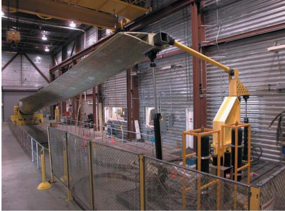
Figure 1. NREL's dual-axis force-displacement fatigue test
