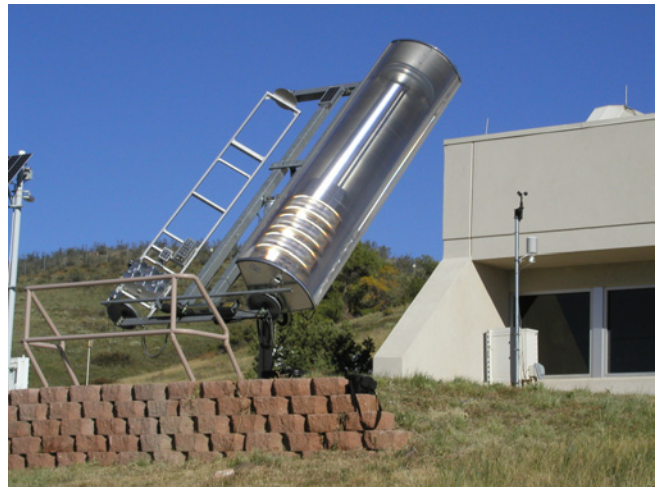
Fig. 2. The OCIV test bed with bare rack on left; enclosed module with primary optics on right.
