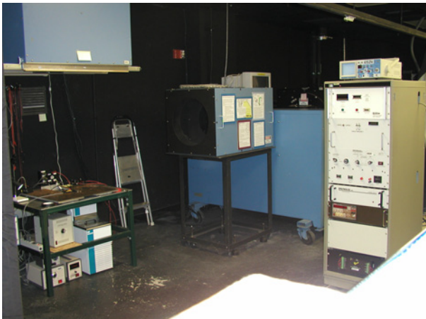
Fig. 1. HIPSS system. Test bed and hood at left, DAQ at right, PFN in middle back.
