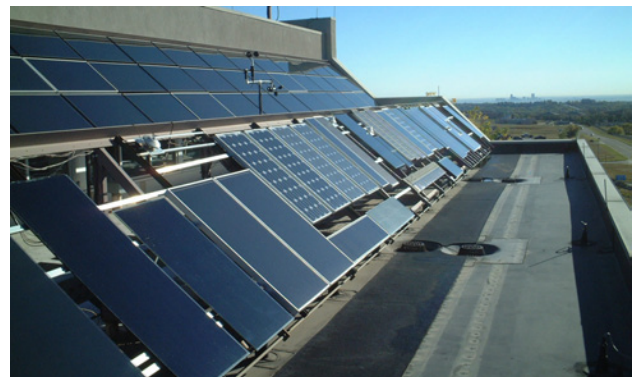
Fig. 2. The Performance and Energy Ratings Testbed on the roof of the NREL Outdoor Test Facility.
