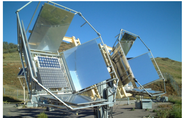
Fig. 1. The Outdoor Accelerated-weathering Test System at the NREL Outdoor Test Facility.
