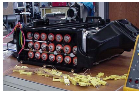
Figure 1, Honda Insight Battery Pack
