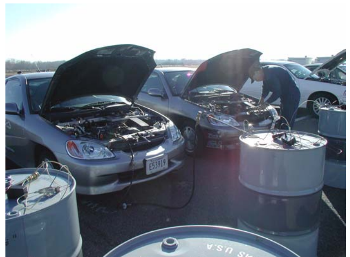
Figure 6. Two Honda Insights Being De-fueled, Flushed, and Refueled
