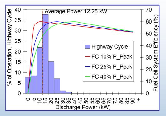
10% peak efficiency FC has the highest fuel economy because its peak efficiency is better aligned with the power requirements.
