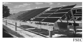
**Figure 5:** Hot and humid testing of thin-film modules at FSEC, Cocoa, Florida
