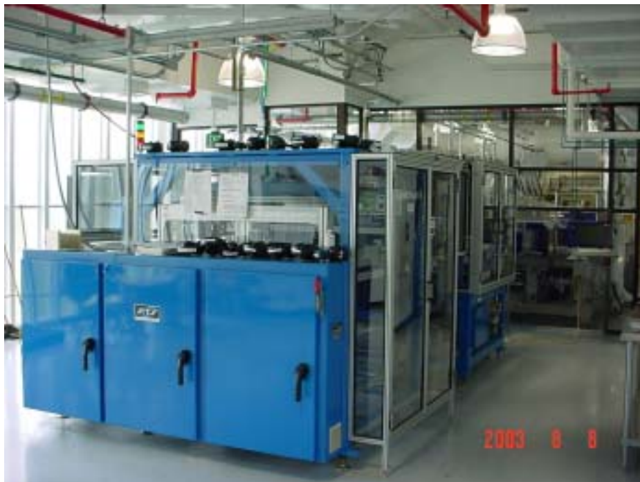
Figure 26: Loading End of In-line Silicon Nitride Equipment - Frederick
