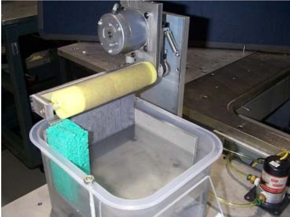
Figure 7: Generation 3 prototype with counter-rotating roller introduced to help wafer singulation
