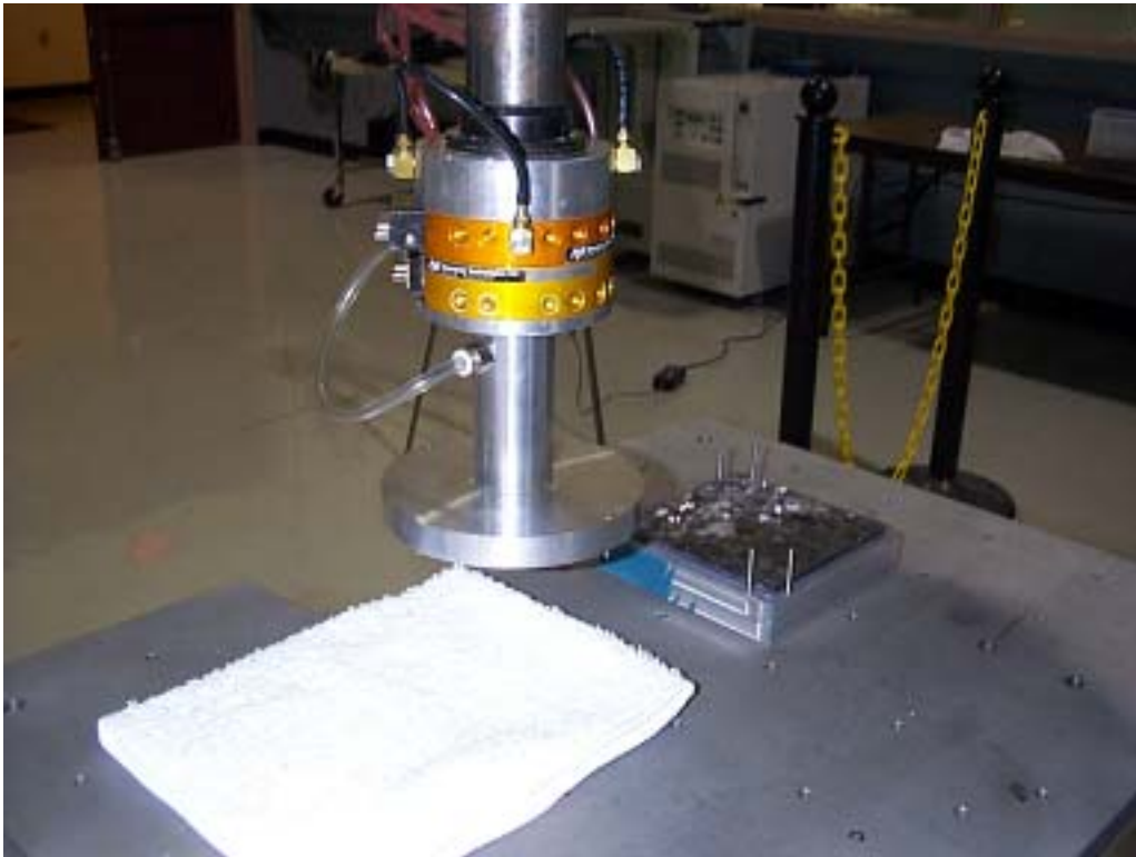
Figure 17: Robotic transfer test of air levitation prototypes
