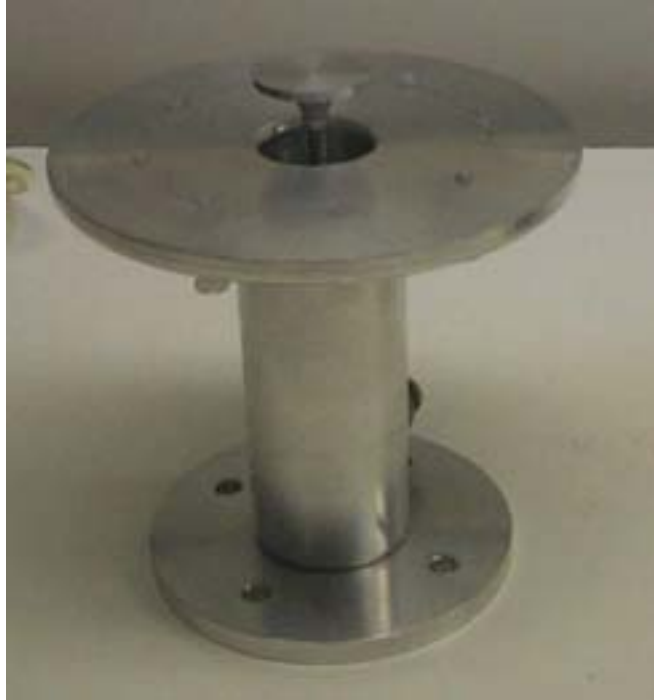
Figure 16: Low-contact valve diffuser design
