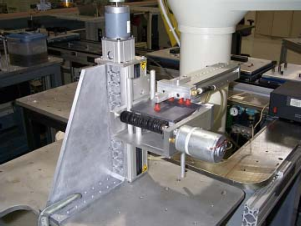
Figure 10: Generation 4 prototype, overall view with step-motor stage for raising the coin stack
