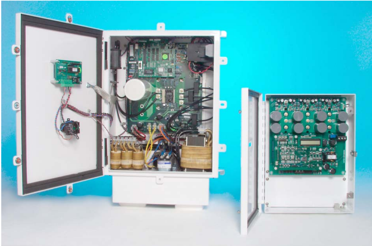
Figure 1. 10kW Inverter Comparison Photograph Left - The existing Xantrex PV10208 Right - The PV10A developed under this contract
