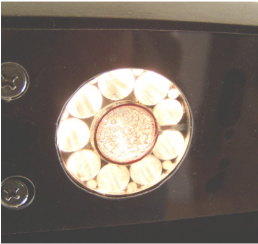
Fig. 15. This sample head is optimized for in-line measurements of wafers or flat surfaces of uniform blocks. The illuminated area is large, to enable high sensitivity for measuring unpassivated wafers just entering the process line, and giving very one-dimensional results on phosphorus-diffused wafers.
