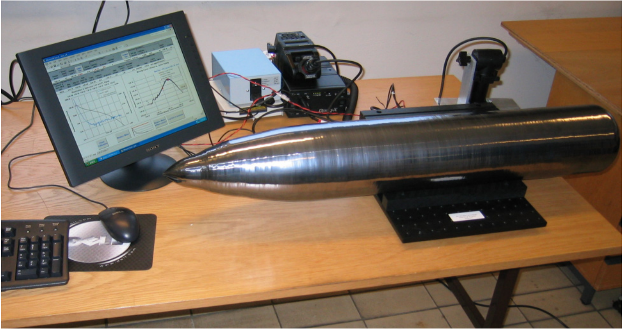
Figure 14. An instrument that was optimized for measurements on as-grown boules of high-lifetime float-zone silicon. (Photograph courtesy of Jan Vedde, Topsil A/S).
