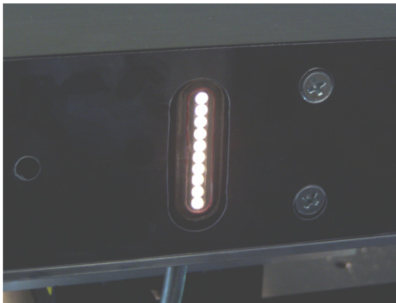
Fig. 9. A detail of the block scanner, the sense head. This spot size is about 3 mm wide, and 30 mm high giving high resolution when stepped in the long (growth) axis of the block. The result is averaged over 30 mm in the axis perpendicular to the growth direction. The total illuminated area is large enough to give very good signal to noise.
