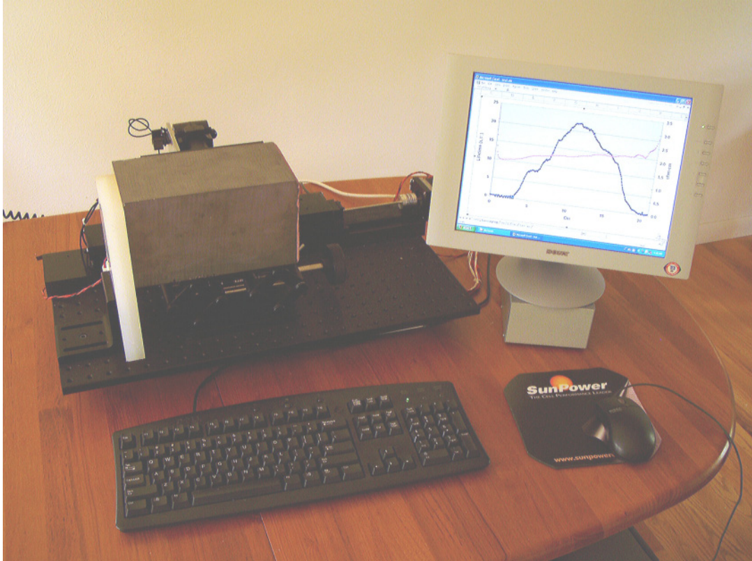
Fig. 8. This instrument performs line scans down the length of a Multi-crystalline silicon block. The sample head, (behind the block) is run along a computer-controlled stage.
