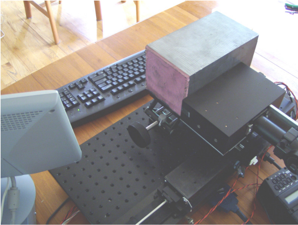
Fig. 10. A different view of the block scanner indicating the sample head as it scans the block.
