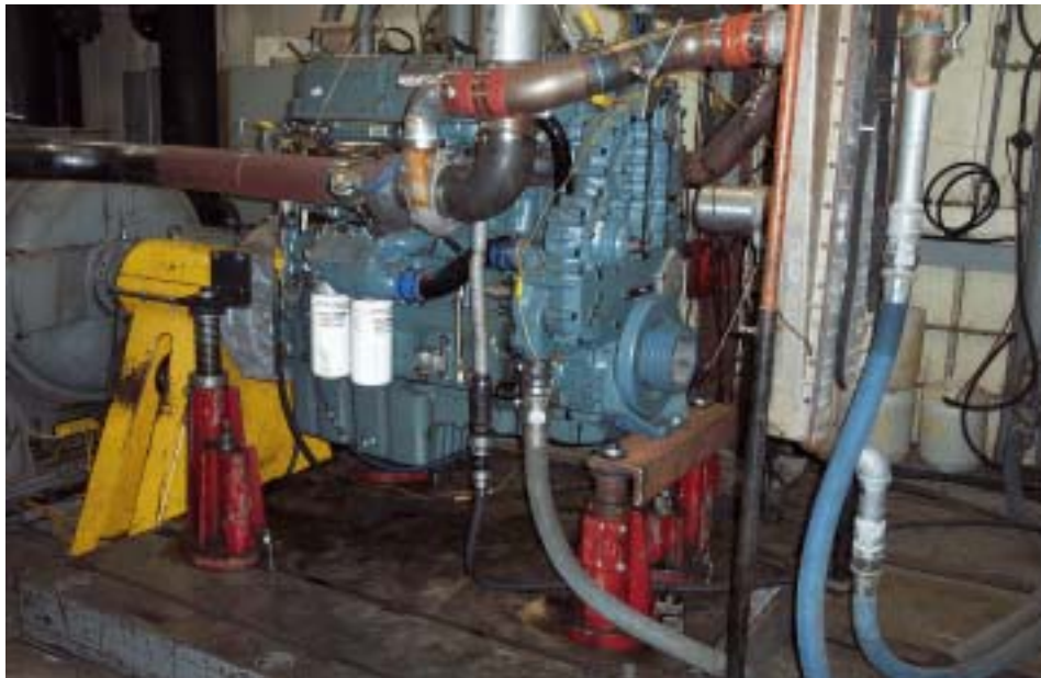
FIGURE 2. DETROIT DIESEL SERIES 60® MOUNTED ON TEST STAND
