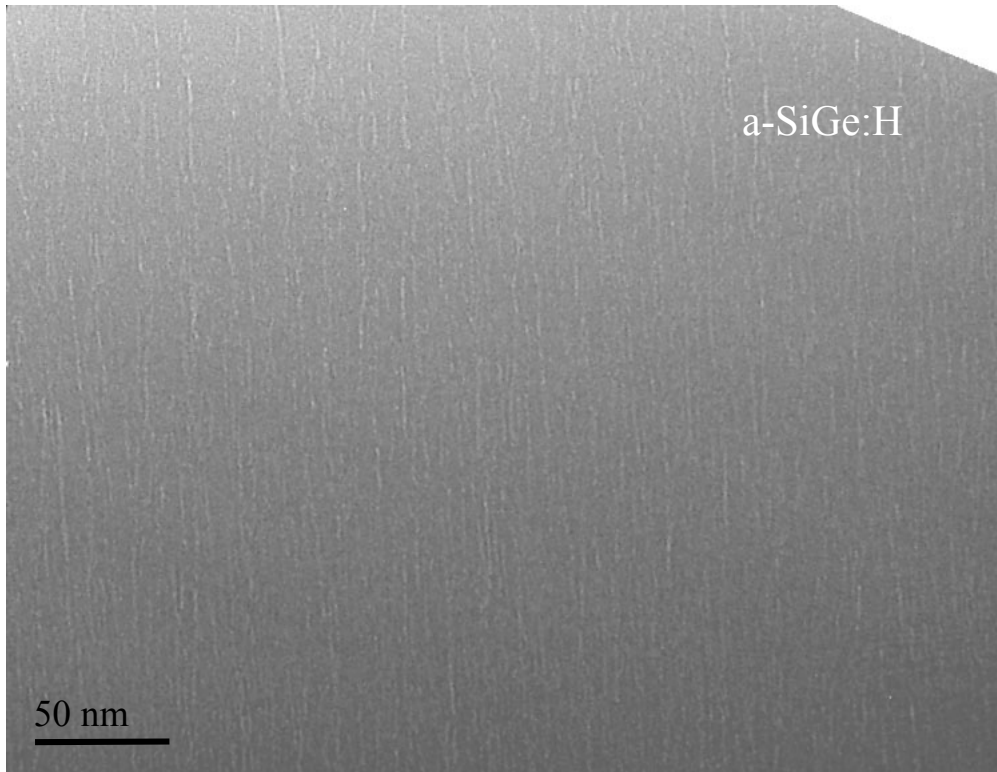
Figure 10. XTEM image showing a large area from a-SiGe:H film (Sample 4, Table 2).
