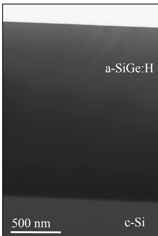
Figure 8. Bright-field XTEM image from the overall HWCVD a-SiGe:H film (Sample 4, Table2).
