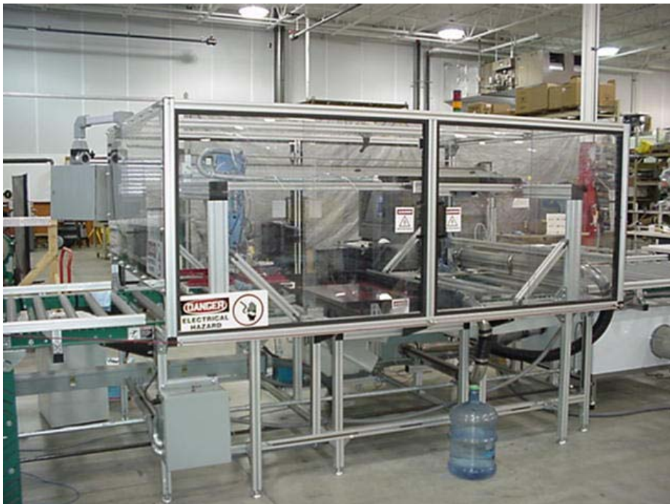
Figure 9. Hi-Pot testing station after lamination
