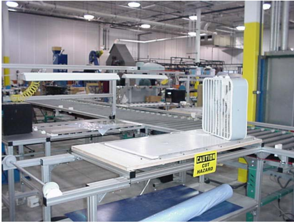
Figure 8. EVA sheet application station before lamination – start of solar finalization line
