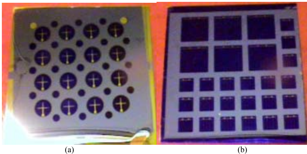
Figure 2B-4 Pattern of ITO and grids with old (a) and new (b) ITO/grids design.
