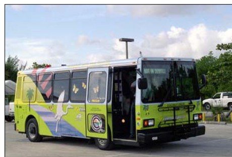
This turbine hybrid bus, operated in Coconut Creek, Florida, is fueled by propane.
