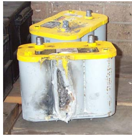
A battery management system could help prevent failure of individual batteries in a pack.
