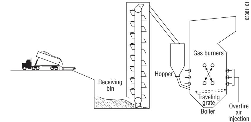
Figure 2. Schematic of a typical traveling-grate spreader-stoker.
