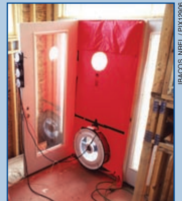
Home airtightness is tested using a blower door.
