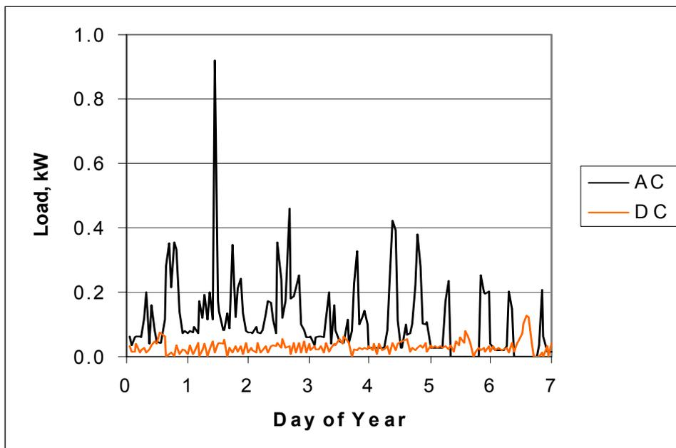
**Figure 6.2. Typical week of hourly average AC and DC load profile**
