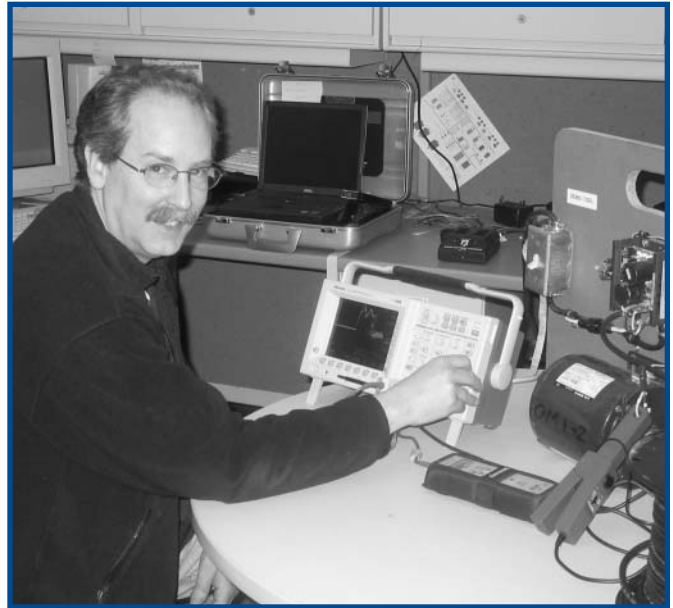
Gary Boyett, Boeing Condition-Based Maintenance Technician, examines the effect of "reflected wave," a potential power quality problem that can be induced upon motors by variable speed drives.
