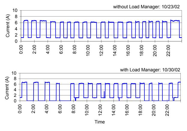
Figure 2: Current profile for vending machine #1 with and without the load manager
