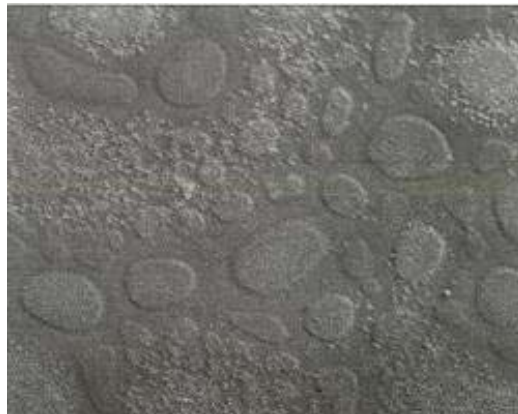
Figure 12.8. Droplet structures on an as-grown Cu-rich \text{CuInSe}_2 film with annealing.
