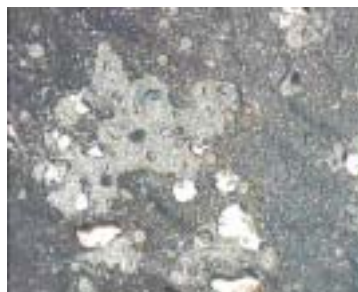
Figure 7.9. Test sample after RTP using a silicon wafer as the susceptor.
