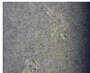
Figure 7.10. Test sample after RTP using a graphite plate as the susceptor.
