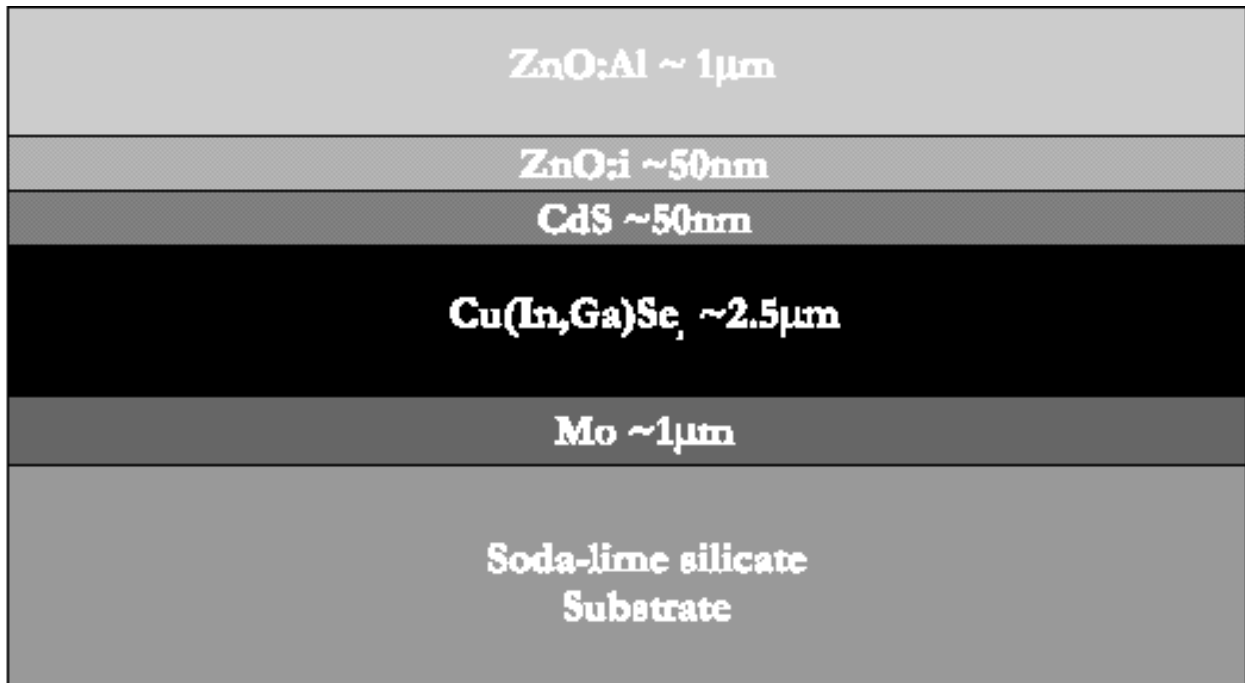
Figure 5.1. Cross-sectional schematic of a CIS solar cell structure.
