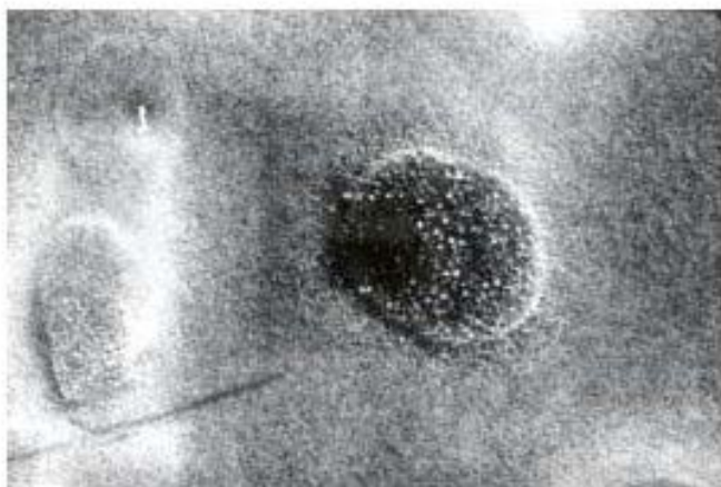
Figure 12.6. Droplet structures on an as-grown Cu-rich \text{CuInSe}_2 film.
